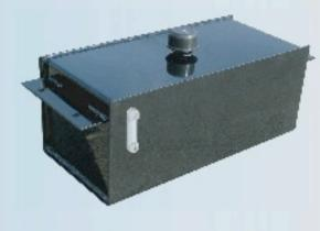
The 8.5 gallon box type reservoir is designed to be frame mounted inframe. It hangs out of the way and is equipped with a brass wire mesh suction strainer, oil level & temperature gauge.
