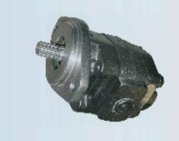
The P22 direct gear pump is bi-rotational with side and rear ports for versatility, thus eliminating the drive line for added safety and dependability. This pump has an S.A.E. "B" 2-bolt flang. 15 GPM @1200 RPM
