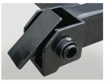
The U720Ds hinges are cast from extra heavy duty 4140 grade steel to ensure durability. Adding to the ease of installation and durability, these hinges are welded directly to the body's longitudinals This Subframe
